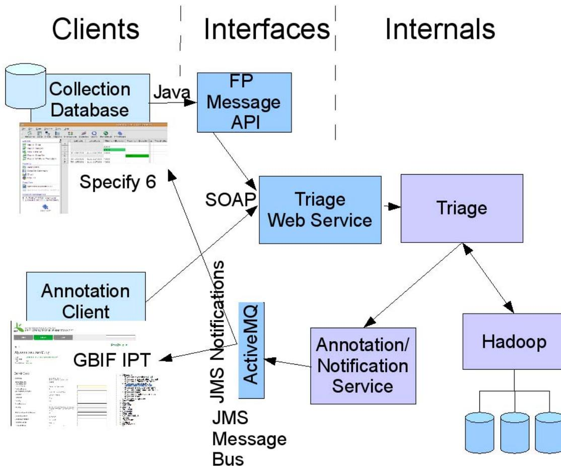
Overview of Clients, Interfaces, and Internals of a Filtered Push network.
