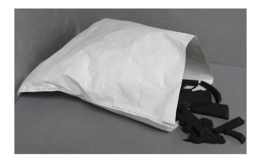
Hang a bag made of Tyvek® under your workbench and gradualy fill with chopped up off cuts of Plastazote™. When full, seal the top and you will have a useful pillow for supporting specimens, while saving waste material from landfill. LAJ
