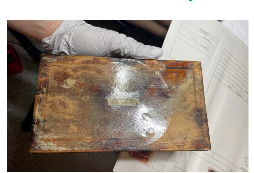
Created for earthquake-prone touring venues to prevent movement of objects. Press a layer of silicone sealant between two sheets of Melinex®, peel the Melinex apart to create two disks of silicone. Allow to cure for 24-48 hours. The disks can then be applied to the base of stable objects and plinths. Areas such as labels can be protected by Melinex. CT1® clear silicone was Oddy tested and passed in 2022. CM
