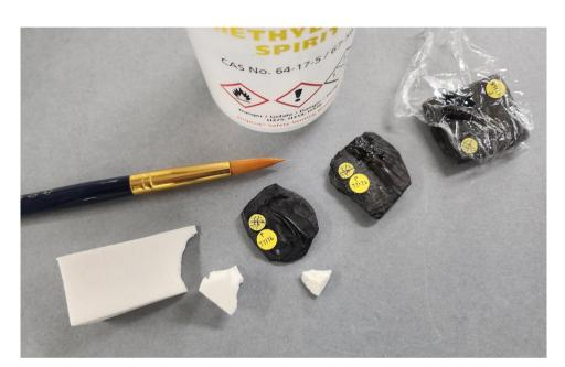
Cosmetic sponge is excellent for removing solvent gels, before clearing with the appropriate solvent. Remember to dab not drag to prevent scratching. LAJ
