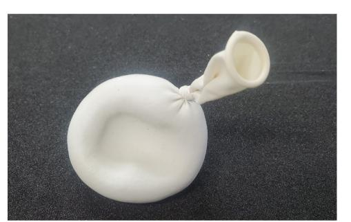
When filled with sand a regular party balloon makes a great temporary supportive sandbag that will hold its shape well when pressed. These can be very handy for supporting awkwardly shaped specicimens when photographing and while adhesives are drying/curing. ER
